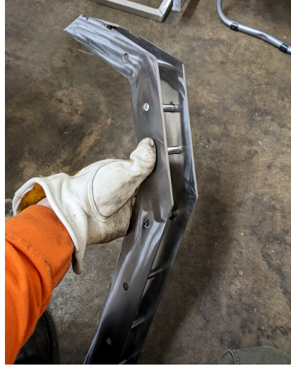
(b) Lower arm sub-assembly, tacked.
