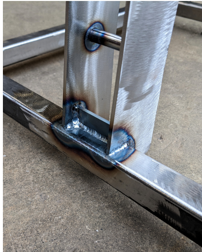
(a) Welds between the arm and frame sub-assemblies.
