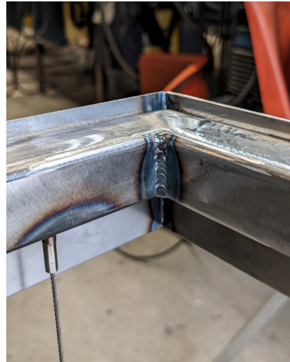
(b) Welds on the upper frame; side skirt interior.
